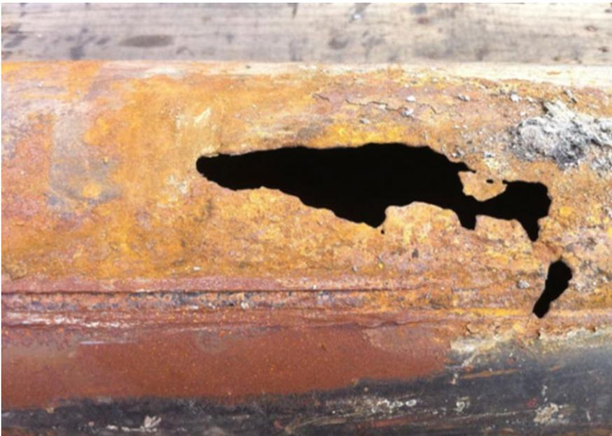
**Figure 8. Corroded tail gas line**
