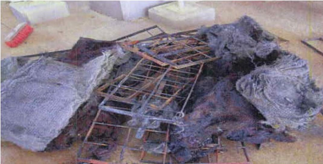
**Figure 2. Damaged demister pads**
