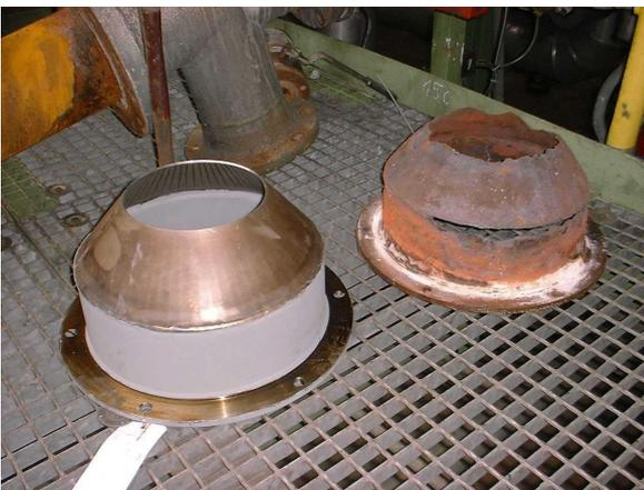
**Figure 3. Undamaged and damaged burner throat**
