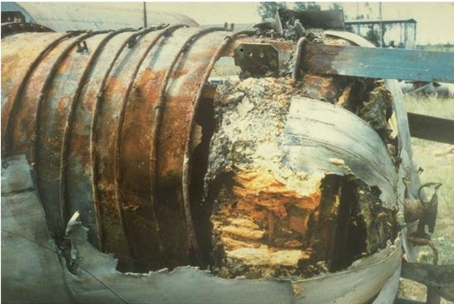
**Figure 15. Coalescer damaged by sulphur fire**
