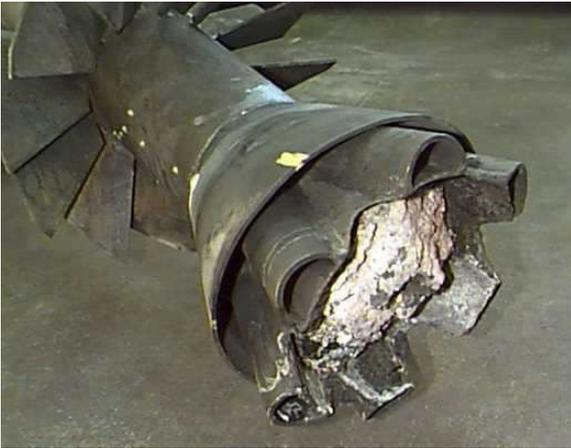
**Figure 2. Burner throat damaged by backfiring**
