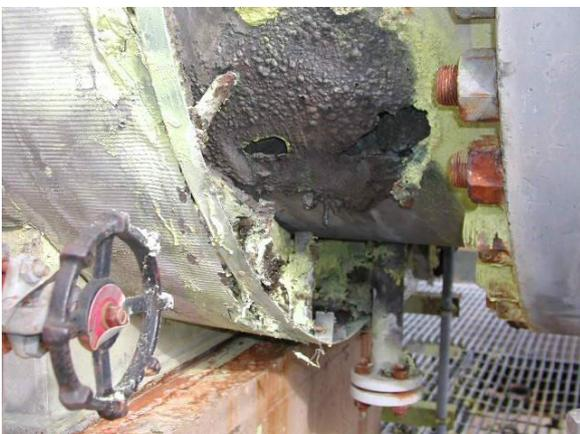
Figure 13. Damaged reheater shell
